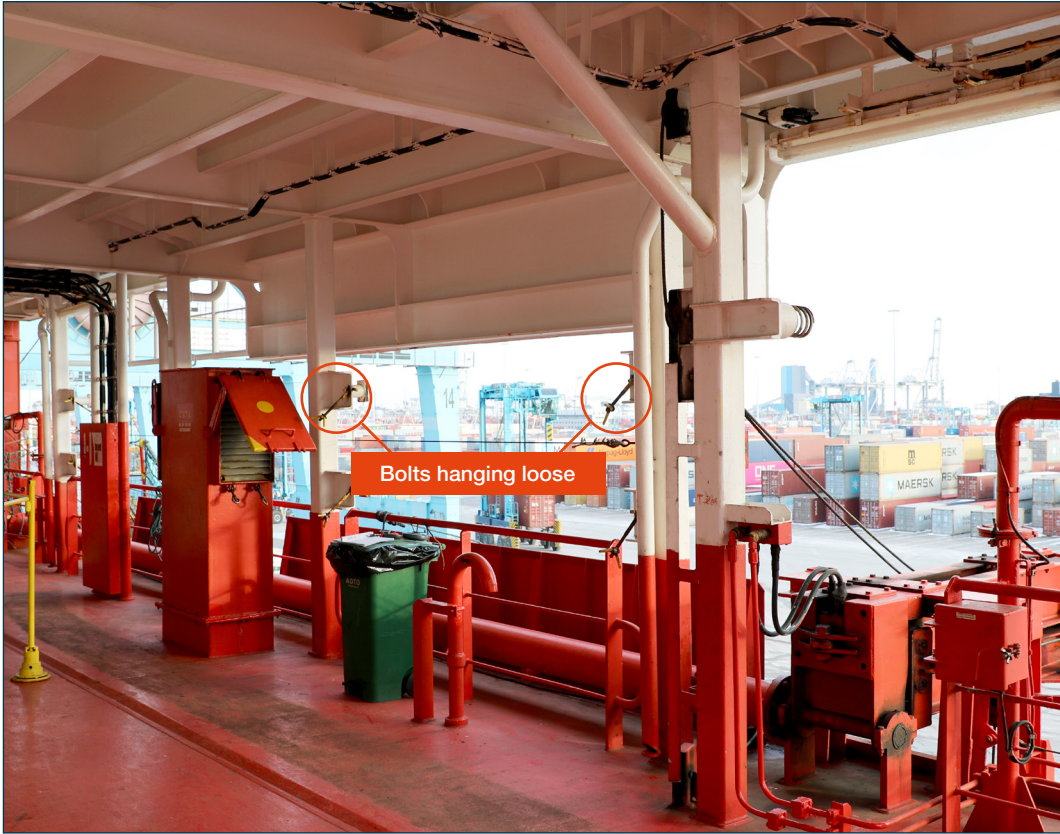
Figure 16: Loose bolt hooks Source: DMAIB
